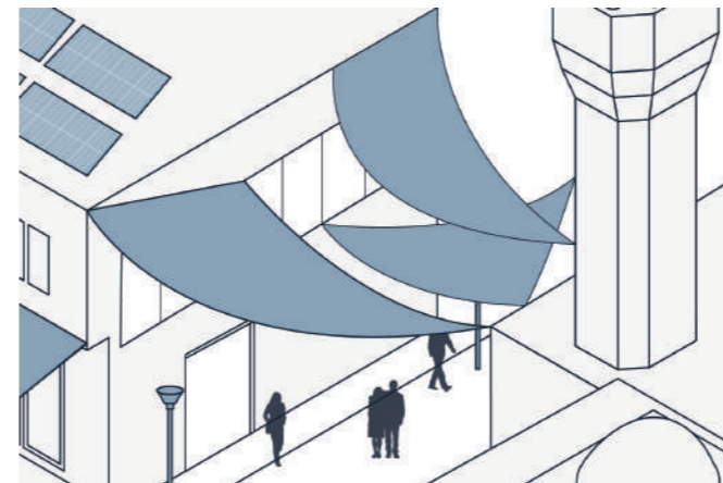
Sails: fabric (or ETF) sails can provide shade in alleyways and contribute to the activation and definition of the space.
