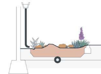
Dry rain garden: Shallow, planted depressions designed to absorb runoff from impervious surfaces such as roofs and pavements or roads.
